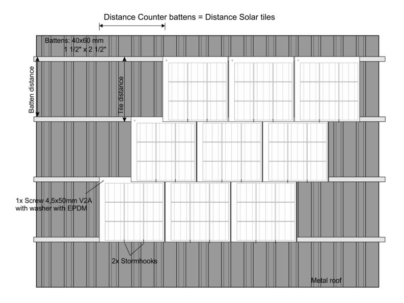
Distance Counter Battens = Distance axis tiles horizontal
