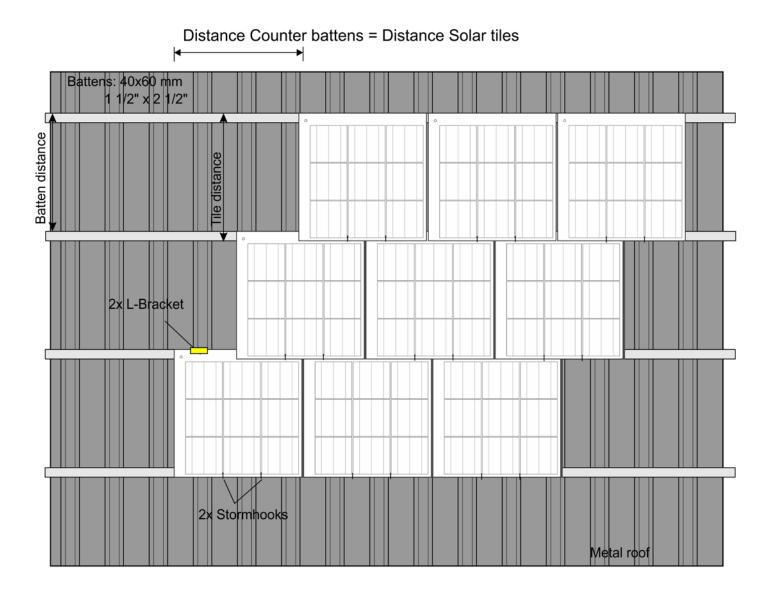
Distance Counter Battens = Distance axis tiles horizontal Minimum: 54.5 cm / 21 1/2"
